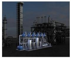
The third generation of high-efficiency absorber, which reduces the unit cost of carbon capture by about 35% compared with the second-generation absorber
