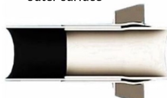
Swaging along the outer surface
